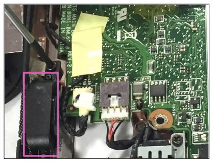
The speakers are located on the right side of the device. There is one speaker towards the top of the device and one on the bottom, just below the volume control buttons.
