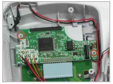
• Use a phillips size #00 screwdriver to remove the two screws, circled in red, from the green circuit board.
