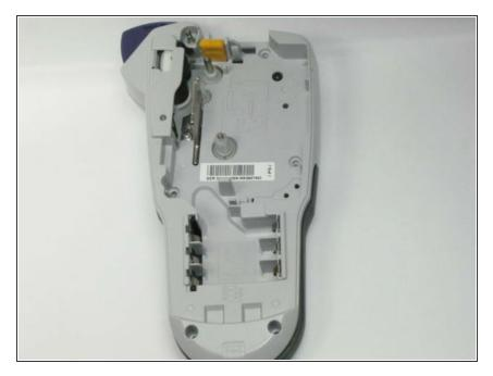
• Remove batteries, cassette tape, and cutter blade.
