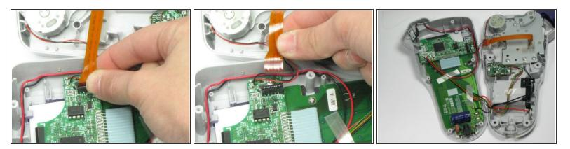
• Using your index finger and thumb, pull out the golden ribbon from the green circuit board.
