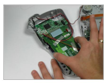
Carefully remove the green circuit board by pulling it straight up. Be careful not to break the LCD cable
