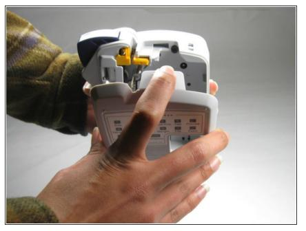
Flip the device over and press down on the indication arrows located at the top center of the back cover and pull it open.
