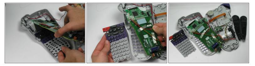
Underneath the circuit board you will find the rubber keyboard. Peel this off and remove it from the device.
