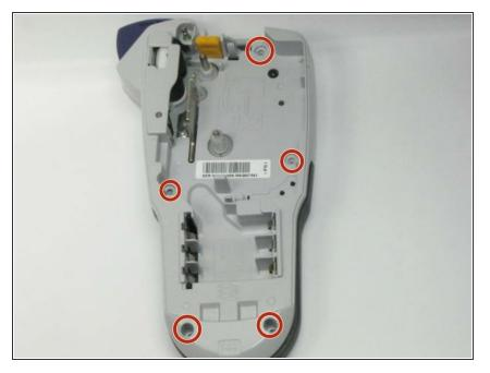
Use a phillips size #00 screwdriver to unscrew the 5 corner screws circled in the picture.
