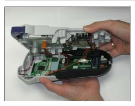
Separate the top of the device from the bottom. Be very cautious when you separate the device, there is a
