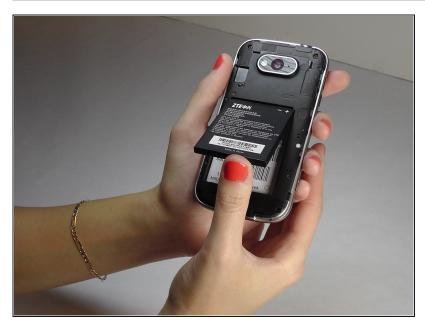
• Pry the battery up and out of the phone.
