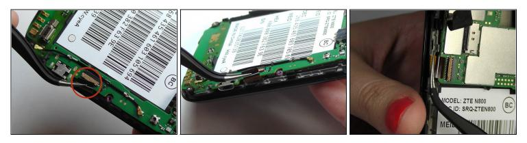
• Use the <u>tweezers</u> to remove the four ribbon wires on the sides of the device.
