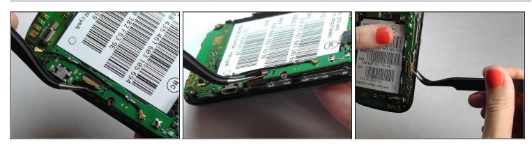
Be careful when removing the ribbon wires. They are delicate.
