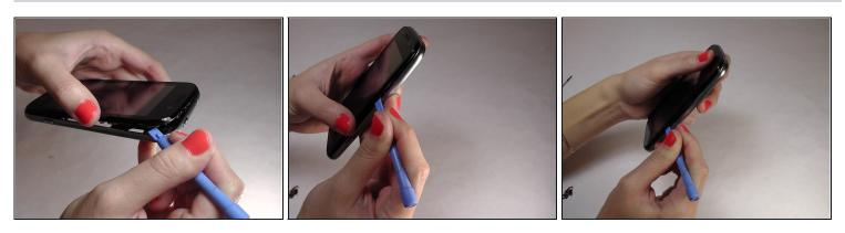
Wedge the flat end of the spudger between the mid frame and the digitizer.
