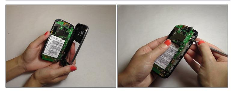
• Gently pry the mid frame away from the rest of the phone to expose the motherboard.
