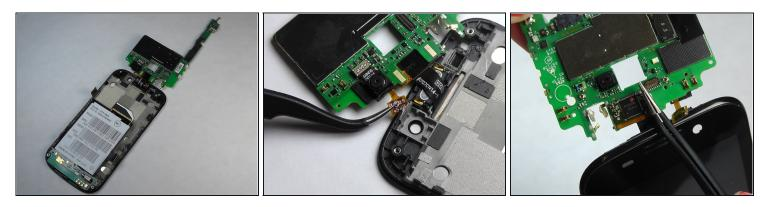
• Remove the remaining two ribbon wires from their connectors.
