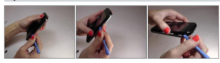
• Gently wedge the spudger in between the glass screen and the mid frame.
