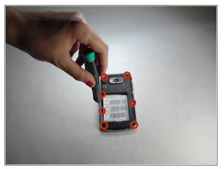
Use the Phillips Head 00 screw driver to unscrew the seven 0.1mm screws from the phone's mid frame.
