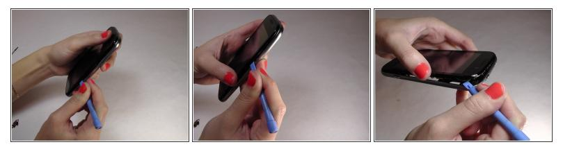
• Gently wedge the spudger in between the glass screen and the mid frame.
