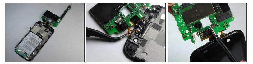
• Remove the remaining two ribbon wires from their connectors.
