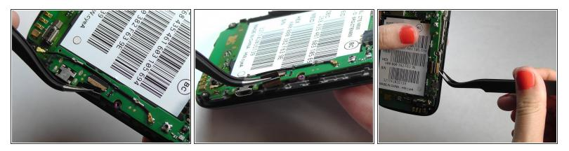
• Be careful when removing the ribbon wires. They are delicate.
