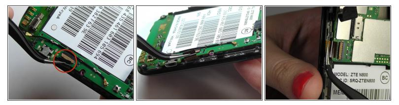
• Use the tweezers to remove the four ribbon wires on the sides of the device.
