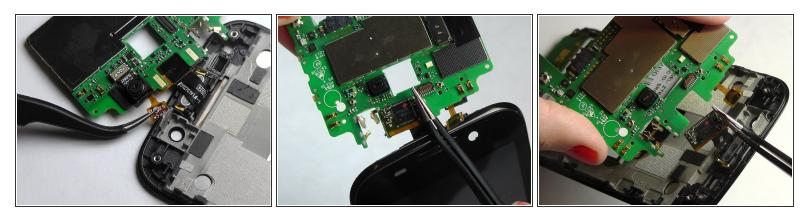
• Remove the connector to free the motherboard from the screen.
