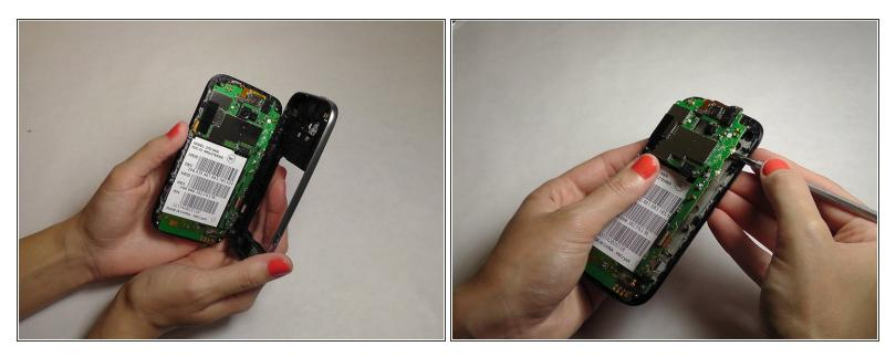
• Gently pry the mid frame away from the rest of the phone to expose the motherboard.
