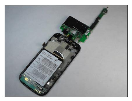
• Orient the motherboard to expose the mid frame.
