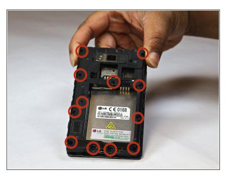
Remove the 12 screws (with the phillips head 000) around frame and near sim and sd cards.
