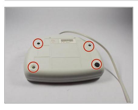
Use a Phillips head #2 screwdriver to remove the four screws from the bottom of the device. These screw heads are sized 5.3mm (or .209").
