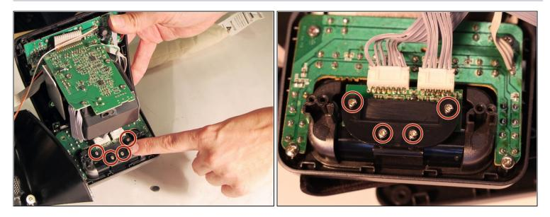
• Remove the four 4mm screws from the protective cover using the iFixit Phillips #1 bit
