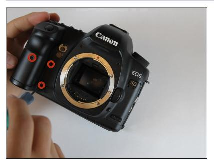
Remove each of the 4.9 mm three screws using a Phillips #0.
