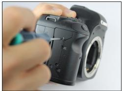
• Remove the four 3.0 mm screws next to the memory card reader using a Phillips #0.
