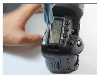
Remove the single 5.9 mm screw next to the the strap loop on the same side as the shutter button.
