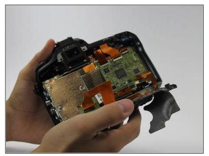
The back panel can now fall off easily by turning the device upside down. Be sure to catch it so the data ribbons do not tear or tug.
