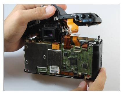
The top panel is now free from the rest of the device. Lift to remove.
