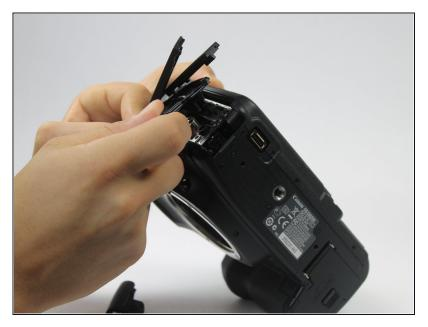
Lift the in/out port plastic covering from the bottom where the backup battery used to be.
