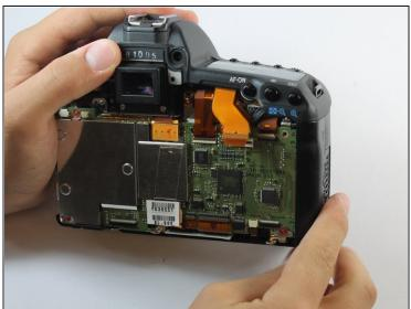
• Using <u>tweezers</u> or your thumb, raise the clasp holding the topmost data ribbon cable in order to release it.
