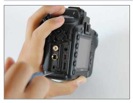
• Using a Phillips #000, remove the single 3.4 mm screw.
