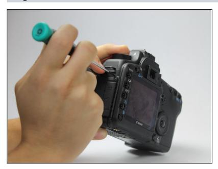
• Remove both 5.4 mm screws using a Phillips #0.
