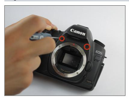
Remove the two 4.8 mm screws above where the lens would be using a Phillips #0.
