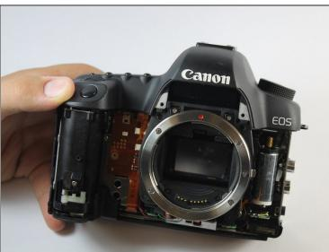
• Remove the front panel by lifting upwards from the right side where the in/out ports used to be.
