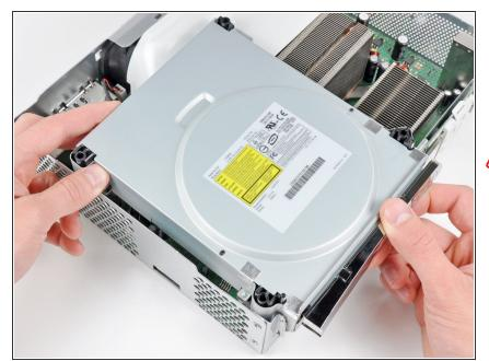
Slightly lift the optical drive upwards to gain clearance to disconnect the SATA and power connectors located on the backside of the optical drive.
