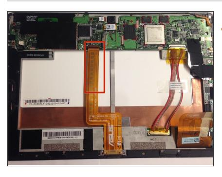
With the battery removed, the charging strip is freely accessible with tweezers. Carefully flip up the white retaining flap on the cable's <u>ZIF connector</u>, and slide the cable out. To reassemble your device, follow these instructions in reverse order.
