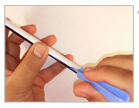
Remove the back cover of the phone with the plastic opening tool.
