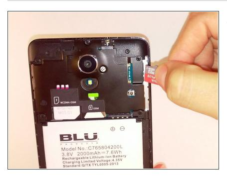
Replace the old memory card by inserting new memory card.
