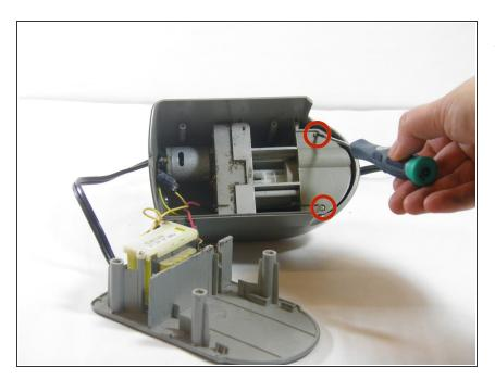
Using a Phillips00 screwdriver, remove two 8.9mm flat edge screws from the top section of the top panel.
