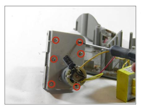
Using a Philips 00 screwdriver, remove the six 9.87mm screws securing the gear housing.
