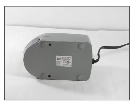
Turn the pencil sharpener on its side.
