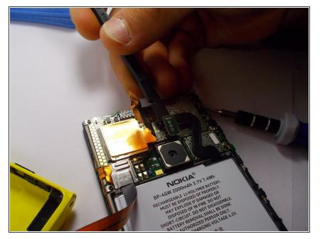
Use a plastic opening tool or spudger, and gently lift up on the connective piece.
