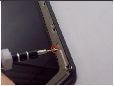
Remove every visible screw tying the chassis to the bottom frame using a T-4 screwdriver bit.
