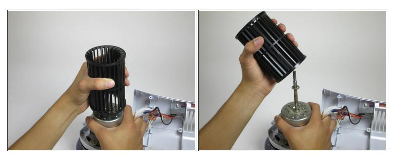
• Grasp the fan blade firmly and pull upward to remove it from the center column of the fan.
