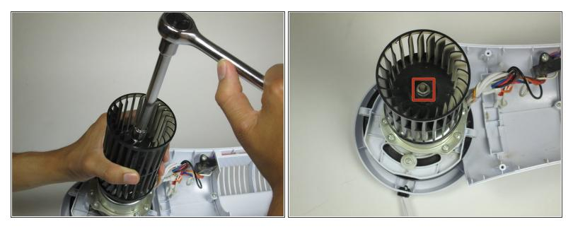
• Remove the hex nut from the fan motor with a 10mm hexagonal ratcheting socket wrench.
