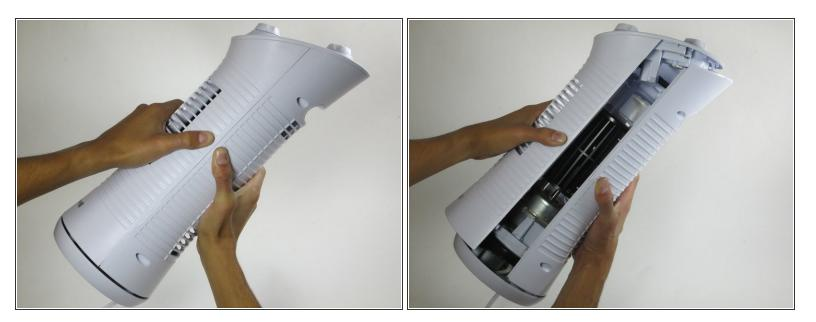
Pull the front and back parts of the case away from each other until the back is free from the front.
