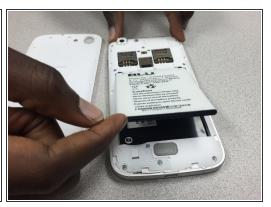
Remove the cover by lifting the notch towards the bottom of the phone. Use your fingernail to lift it up.
