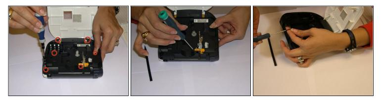
• Remove all 1/4 inch screws(6 total) with a (+PH00) screwdriver. Open slowly not to damage the display data cable.
