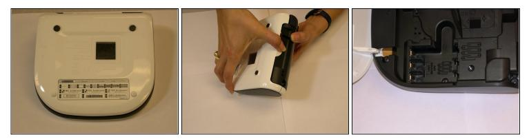
• Turn the device to it's side toward the bottom of the keyboard. Then pop open the case and remove the batteries.
