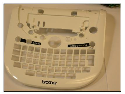
• Change out old damaged face plate with your new face plate.
