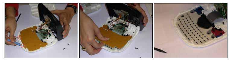
• Use a plastic opening tool to remove the flat-panel membrane keyboard. Lift up and set aside.
