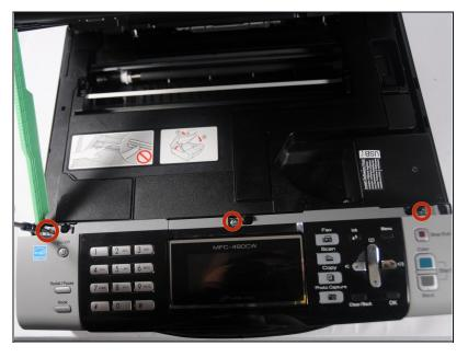
Use a Phillips #2 screwdriver to remove the three 12.1 mm screws holding the control panel in place.
