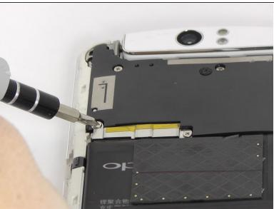
Remove the six 4mm long screws holding the motherboard in with the ph0 Phillips head screw driver.
