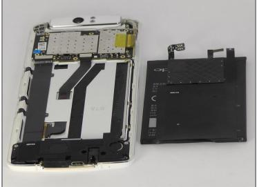
• Use the blue opening tool to carefully pry the battery from the sticky tape that attaches it to the device.
