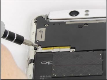
• Remove the six 4mm long screws holding the motherboard in with the ph0 Phillips head screw driver.
