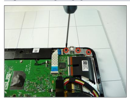
Locate and remove three Phillips screws
