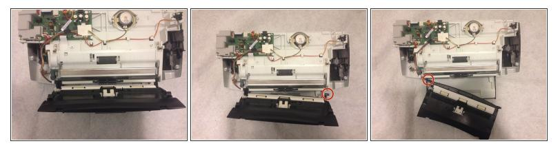
• Pull off the entire black front panel (where the motherboard rest on) by unfolding it forward (as if you're fixing a paper jam) and pull it forward until it pops off.
