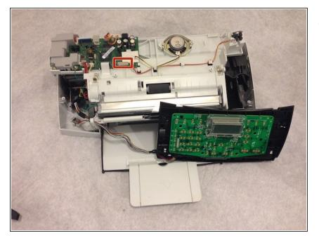
Follow the wires from the left side of the keypad motherboard (on the panel you just removed) to the main motherboard and carefully unplug the wires from the main motherboard (located in the upper left corner.)
