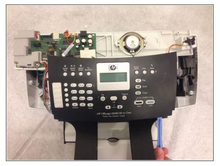
Using the plastic opening tool, Pry off the front black plastic panel on screen area. This panel has the HP symbol on the front.
