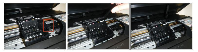
Lift the lever located on the right side of the printhead.
