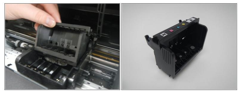
Lift the printhead and remove it.
