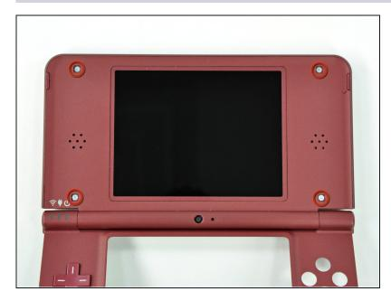
• Remove the four 3.5 mm silver Phillips screws securing the rear bezel to the front bezel.
