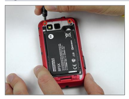
Unscrew the two silver screws located at the top of the back of the phone.
