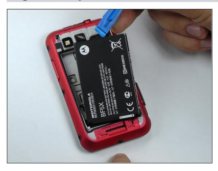
Use a plastic opening tool to pry the battery out of the phone.
