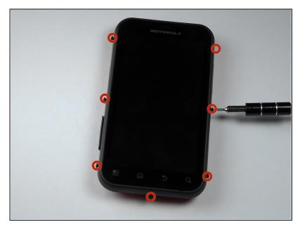
Using the screwdriver and the T-5 bit, unscrew the seven 5 mm screws around the outside of the phone.
