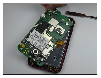
The motherboard is the whole green board. Pry it off carefully with tweezers from the sides and place it aside.
