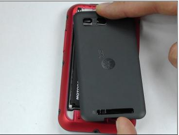
• Remove the back cover of the phone by sliding the bottom black button to the unlock position and lifting it up.
