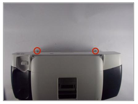
Using your Torx T10 screwdriver, remove the screws indicated in the picture. Screws are 13mm in length.
