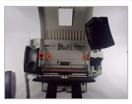
Using your Torx T10 screwdriver, remove the screws indicated in the picture. Screws are 13mm in length.
