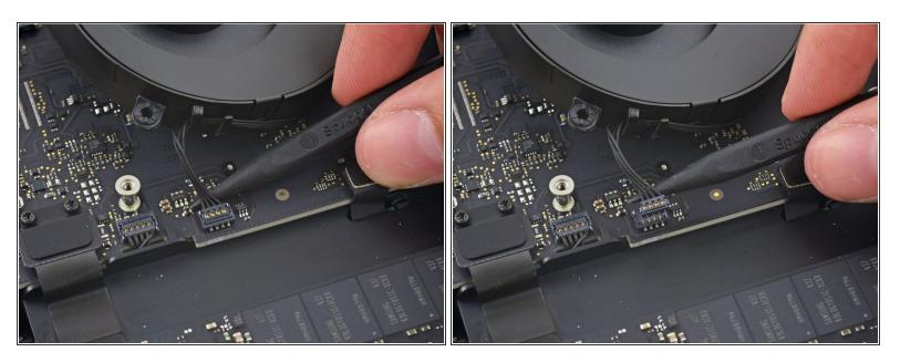
Use the point of a spudger to lift the fan connector straight up out of its socket on the logic board.
