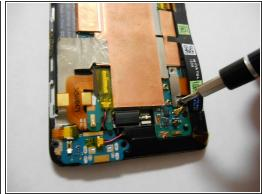
• Remove the two Phillips screws securing the battery connector.
