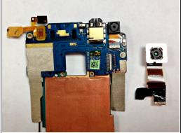
• Use the tweezers to lift the hatch and remove the part of the rear camera that is inserted.
