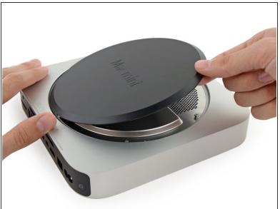
Lift and remove the bottom cover.
