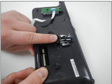
• Push forward and down to release the retaining piece. This will detach the display screen from the front panel.
