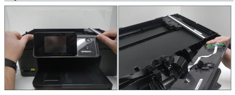
Place thumb and forefinger where shown and pull this piece away from the printer.
