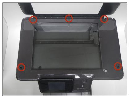
Using the T9 Torx Security screwdriver bit, unscrew the five 12mm screws shown.
