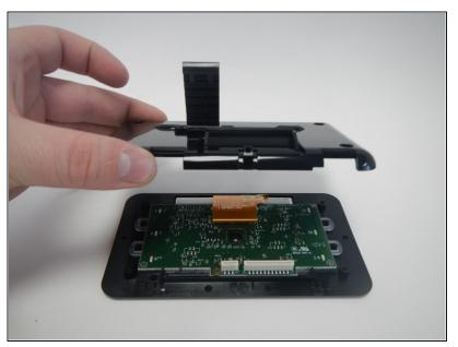
• Lift the back of the display screen to remove it.
