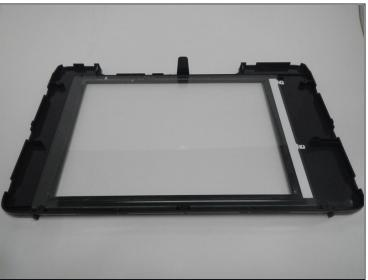
• Lift the scanner glass piece from the printer and set it aside.
