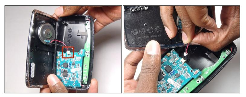
Carefully detach the wire running from the speaker to the motherboard by unplugging it from the white socket.
