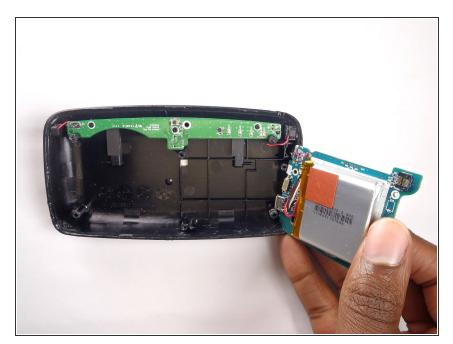
Remove the motherboard from the device by lifting it up from the back plate.
