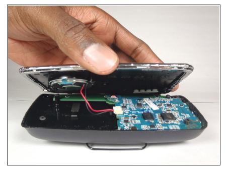
Open up the device by pulling the front plate straight up from the back plate.
