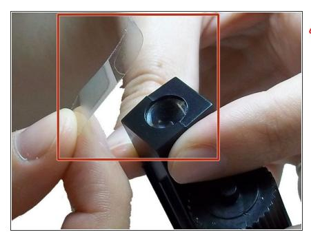
Apply tape to the lens for safe removal and prevention of injury.
