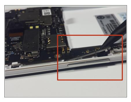
Use the sharp end of the spudger to pry the volume button bracket from the side of the rear case.
