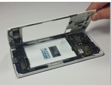
• Insert the plastic opening tool underneath the chassis near the power button and pry the chassis from the phone. This should take a little force.
