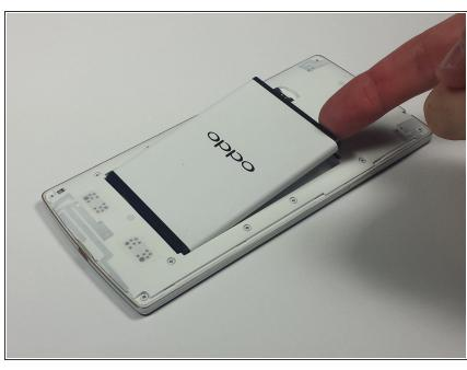
With your finger, remove the battery from the phone by gently lifting the top-right corner nearest to the camera.
