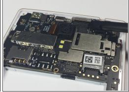
Using the flat end of the spudger, pry the four tape connectors straight up out of their respective motherboard sockets.
