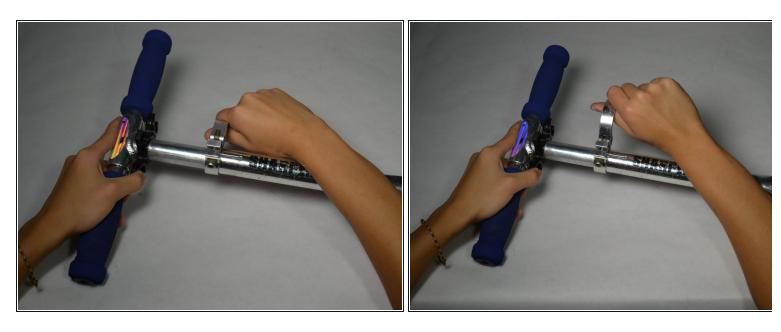
• Unlock the quick-release lever by turning the lever from a tightened position.
