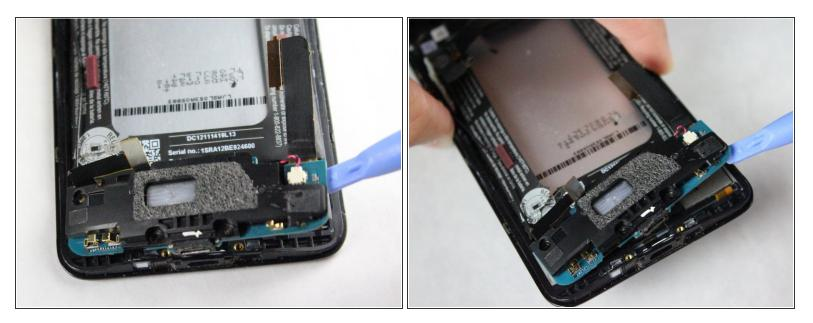
• Use the plastic prying tool to gently remove the charging port assembly.
