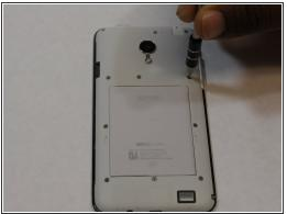
Using one of the small Phillips screwdriver bits provided unscrew the 11 screws present on the protective plastic plate under the device case.
