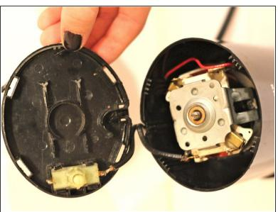
Work your way around the four clips, loosening each a little at a time. Eventually, all four clips will be loose enough to remove the base plate.
