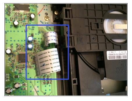
Locate and gently remove the data strips on the tray. There are three in total, two on the left hand side and one on the right.
