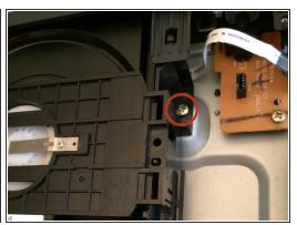
As noted by the red circles, locate and remove the screws one at a time
