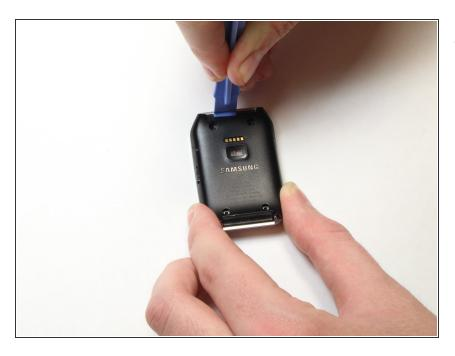
Gently work the plastic opening tool under the top edge of the watch's back cover.
