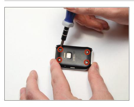
With the watch laying face-down, locate the four screws. They are located on the back of the watch, at the four corners.
