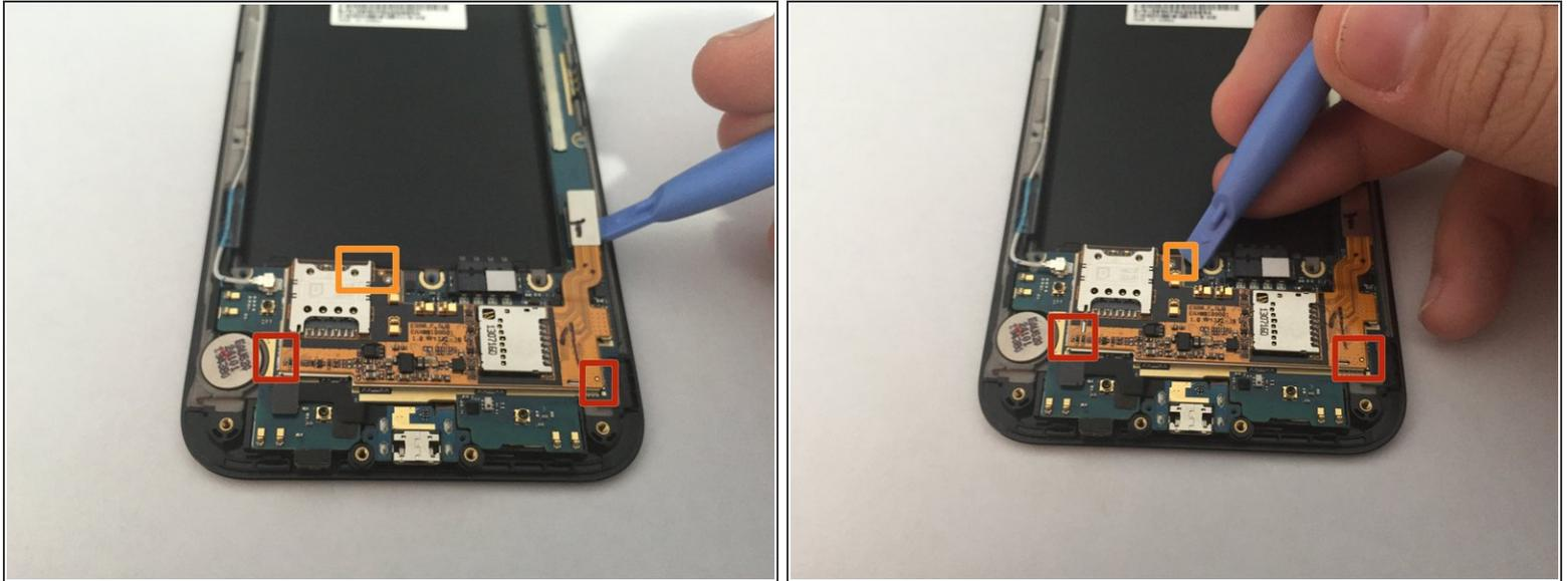
**!** In this next step it is easy to pry the wrong piece. Make sure to pry at the metal platform that the sister board sits on, not the orange printed circuit board itself.
