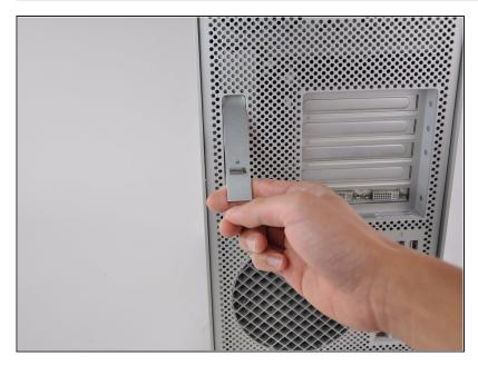
• Lift the lever to unlock the case.
