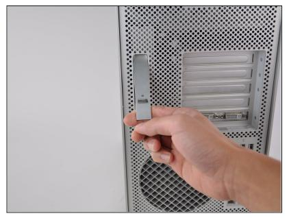
• Lift the lever to unlock the case.
