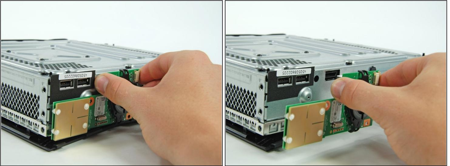
ⓘ The RF module is still connected to the Xbox by a large USB-type connector.
