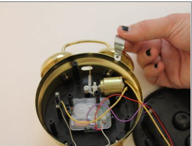
Carefully remove the silver brace which is located on top of the cylindrical solenoid. Set aside.
