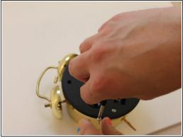
Using the 26 bit driver kit, use the PH1 screwdriver bit to remove the three gold screws from the black plastic back plate from the alarm clock.
