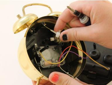
Using the mini screwdriver remove the silver screw located within the white plastic post located on the right side of the solenoid and remove the striker from the bottom of the oval opening which is located on the top of the alarm clock.
