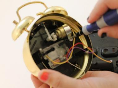
The solenoid is located in the upper right corner of the alarm clock and is supported by a silver brace. Using the screwdriver remove the silver screw from the silver brace supporting the solenoid. Set the silver brace aside.
