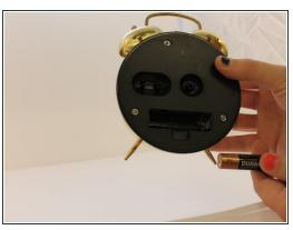
Remove battery cover using the 26 bit driver kit with the #030 bit screwdriver or use thumbnail into indentation within the battery cover. Proceed with the removal of the battery. Set battery and battery cover aside.
