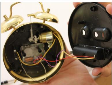
Carefully lift the black plastic back plate away from the alarm main component.
