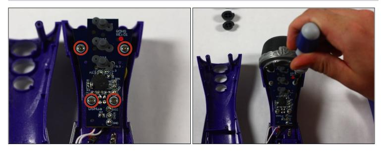
• Remove the 2, #8 11.7 mm Phillips Head screws as well as the 2, #8 7.5 mm screws on the printed circuit board.
