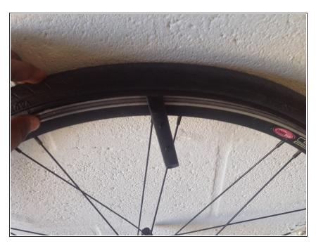
Reattach the the first lever to the other side of the tire and repeat steps 4-7 to remove tire completely from rim.
