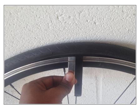
Insert a second tire lever next to the first lever to create leverage for releasing the tire from the rim.
