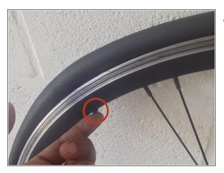
• Push the valve stem upwards through the hole in the rim.
