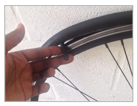
• Once valve stem is pushed, pull the inner tube until it is completely removed from the rim.
