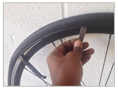
• Leave the first lever in place. Slide the second lever against the outside edge of the rim until one side of the tire is off of the rim.
