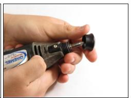
• Remove the black housing cap from the Multipro located directly below the chuck cap.
