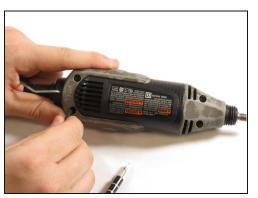
• Remove the 4 screws located on the bottom of the Multipro with a T15 screwdriver.
