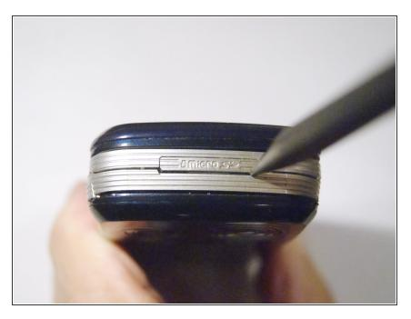
Lift the MicroSD card cover up from where the spudger is pointed.
