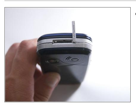
Remove MicroSD card from exposed slot.
