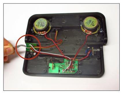
Use tweezers to carefully place the newly soldered Line In chip back into its original position.
