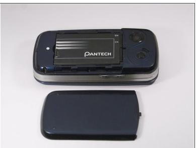
Gently slide the backside phone cover off exposing the battery underneath.
