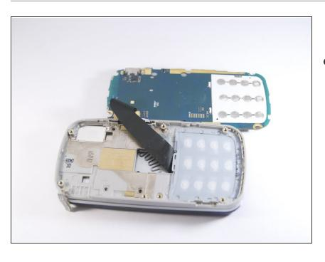
Carefully lift up the motherboard to expose the back of the keypad.
